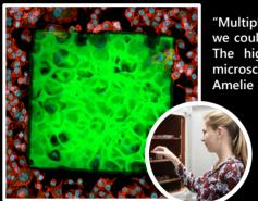
"Multiphoton imaging with the MPX allows us to image our 3D tissue-engineered constructs. Here, we could image a cell-seeded nanoscribed 3D-printed lung tissue scaffold of 300 x 300 x 300 μm. The high penetration depth combined with the intrinsic confocal features of multiphoton microscopy makes it a suitable tool for us to image our samples" Amelie Erben, PhD student
